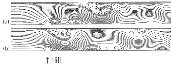
Fig. 12. Instantaneous streamlines around a hill for K = 1.5 , Re = 2000 : (a) Low- C_d state, t = 314 ; (b) High- C_d state, t = 339 .
